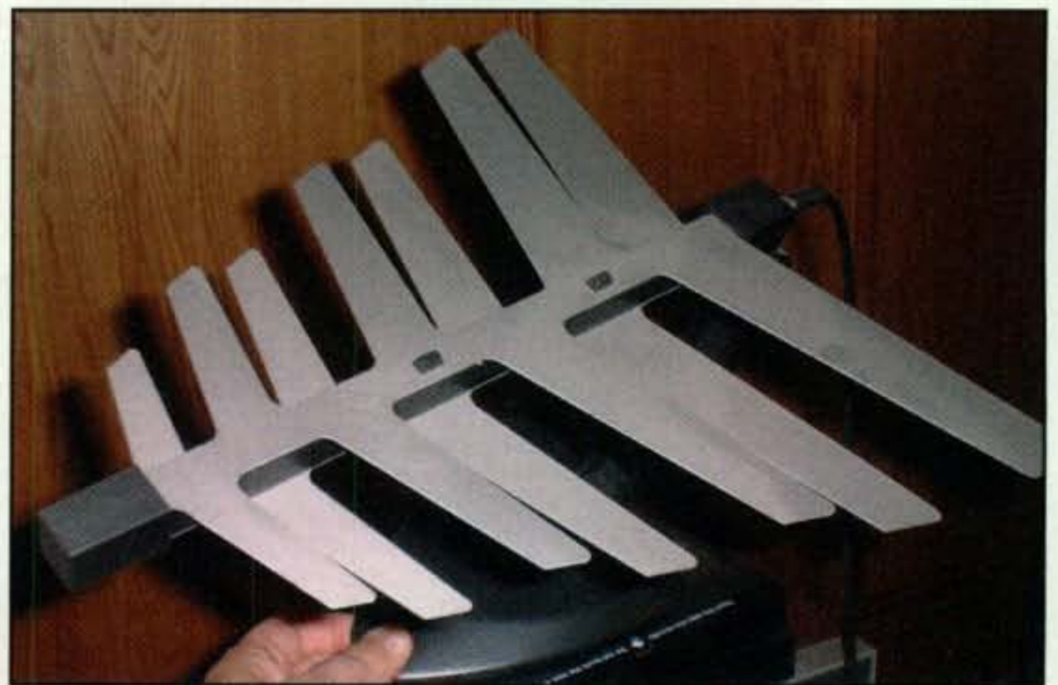
Photo B— Properly phased log-periodic elements.
